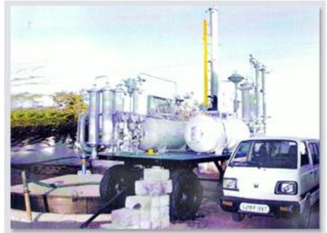
By an approximate formula, 100 cows will give/day 1000/Kg of cow dung, this in a bio digester will yield about 40 M3 of Gobar gas. After removing impurities such as CO<sub>2</sub>, Sulphur, Moisture etc will yield about 20M3 or 17Kg of pure methane gas.
